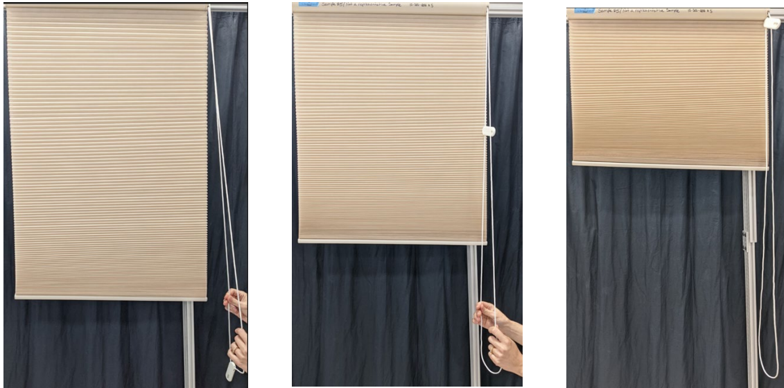
Figure 23. Partially operable window covering when tension device is not attached to a fixed surface
