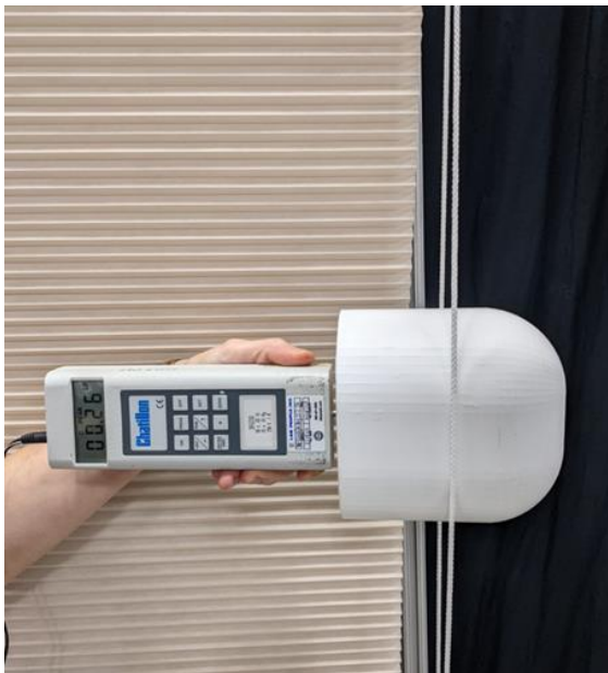
Figure 2. A head probe can pass through properly installed continuous loop under tension.
