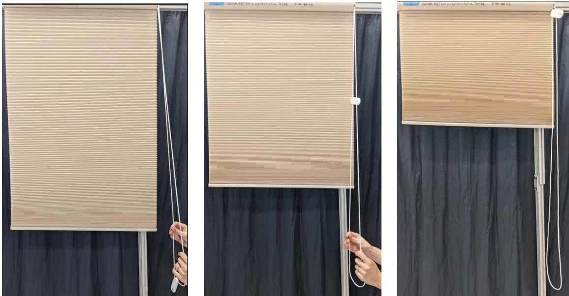
Figure 3. Partially operable window covering when tension device is not attached to a fixed surface.
