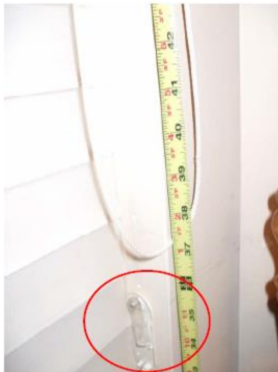
Figure 11. Photograph from IDI 140203CCC2348 shows the incident blind with the broken tension device and exposed cord loop.
