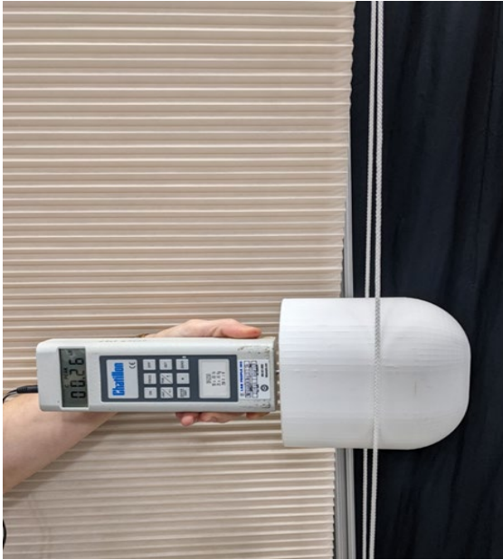
Figure 21. A head probe can pass through properly installed continuous loop under tension
