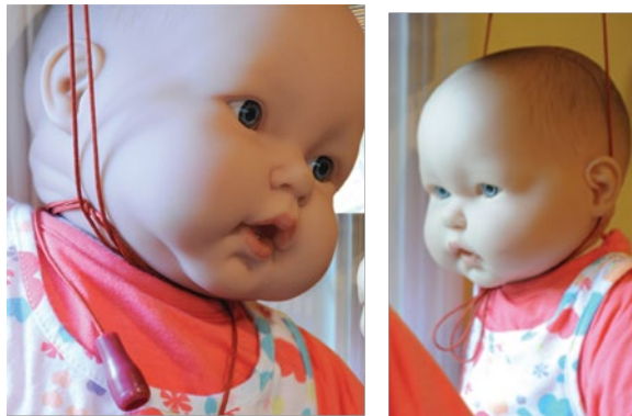
Figure 13. Demonstration of wrapped cords around (doll) child's neck (left), (doll) child's head is through the loop created by entangled multiple cords (right)
