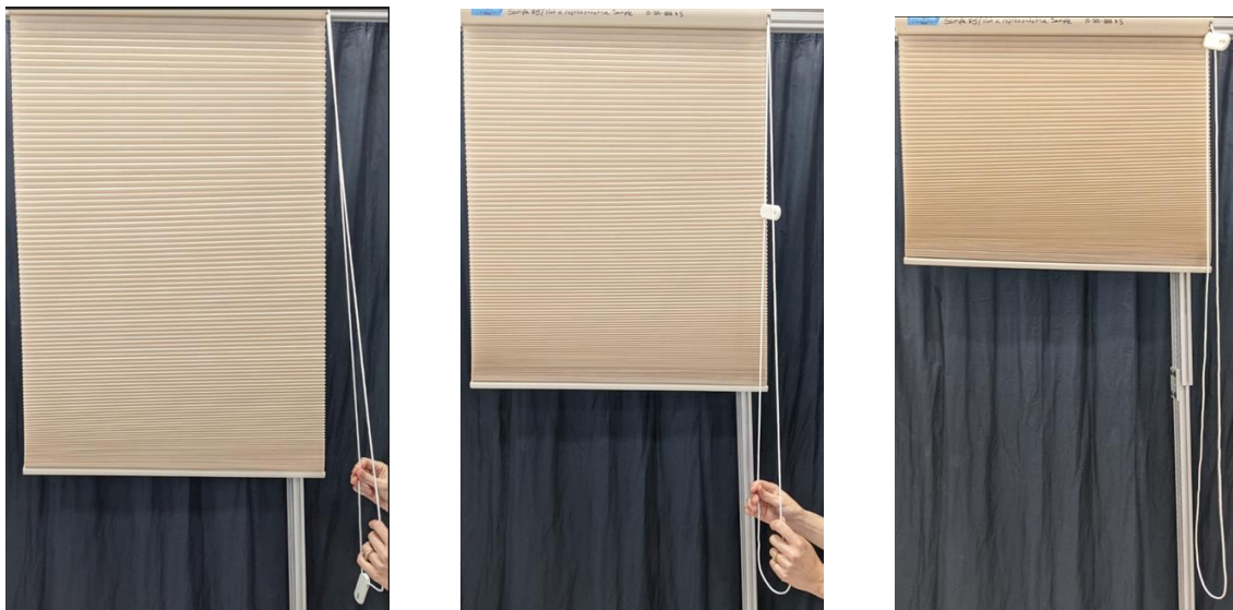
Figure 4. Partially operable window covering when tension device is not attached to a fixed surface.
