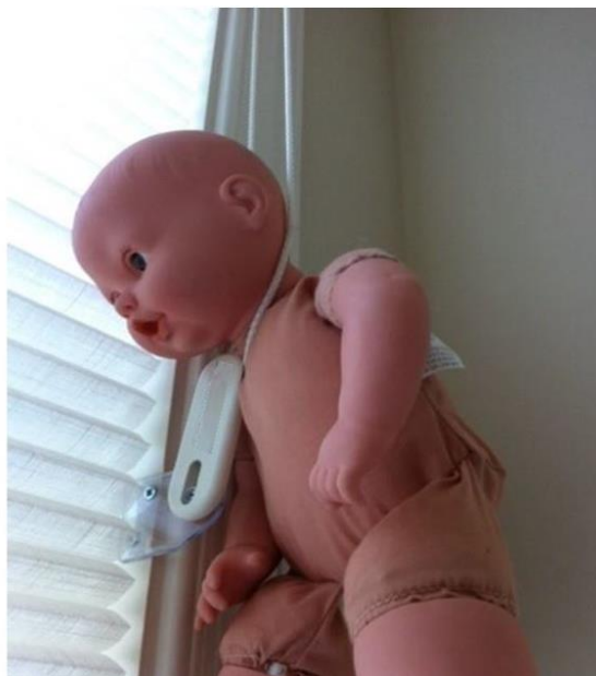
Figure 3. Re-enactment of how a 5-year-old child was found by a consumer with his head caught in a continuous cord loop.
